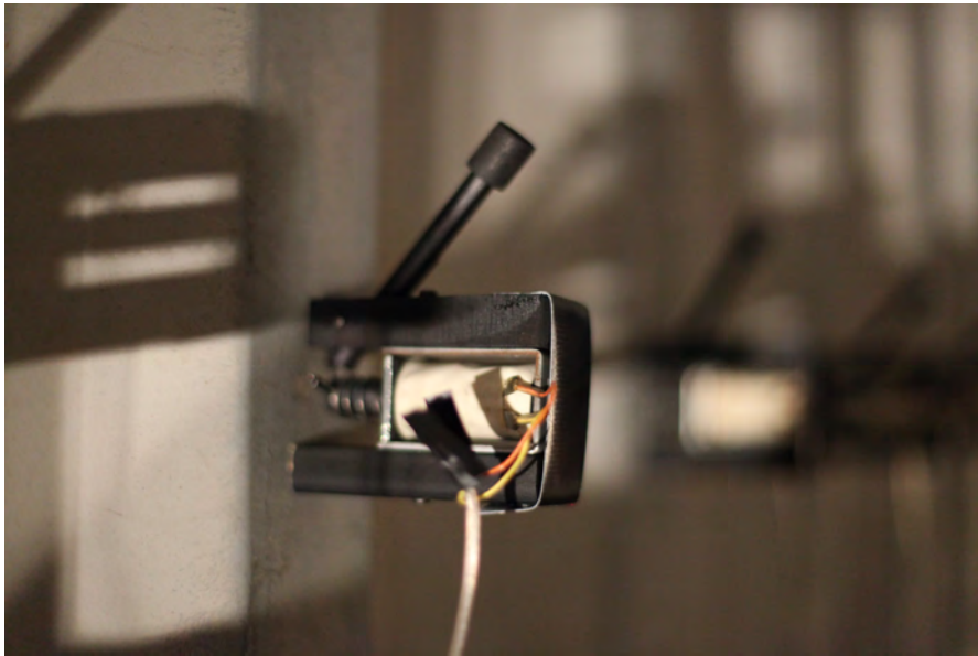
Figure 6.8: Solenoid mounted on the wall of the container.
