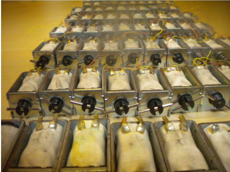
Figure B.9: Twenty-four volt solenoids.
