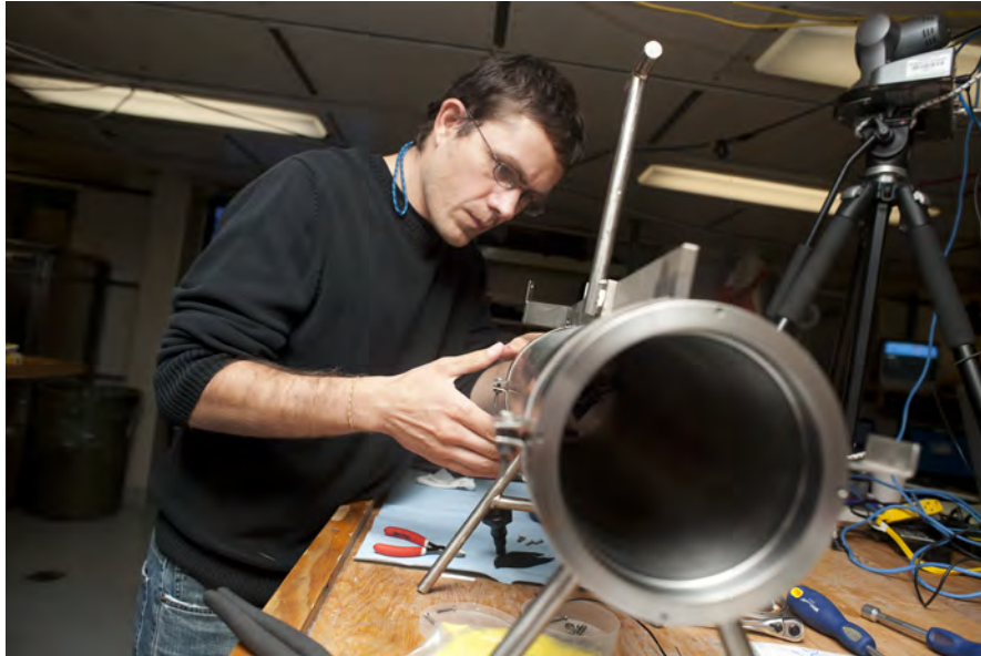
Figure 5.15: Preparation of recorders, placing two recorders inside the pressurized host.
